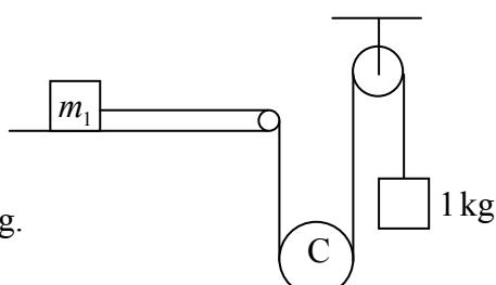
The string then passes over a smooth fixed pulley and supports a mass of 1 kg.
