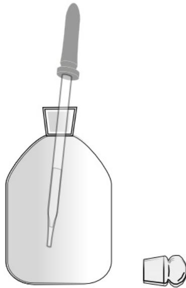
After the three additions, the thoroughly mixed contents of the sample bottle were titrated in 200 cm<sup>3</sup> portions with a 0.02 M solution of sodium thiosulfate (Na<sub>2</sub>S<sub>2</sub>O<sub>3</sub>). The average titre was 9.4 cm<sup>3</sup>.
