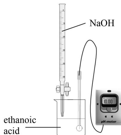
A sodium hydroxide solution was titrated with a solution of ethanoic acid using the apparatus shown on the right. A number of pH readings, together with the corresponding volumes of sodium hydroxide solution added, are shown in the table.
